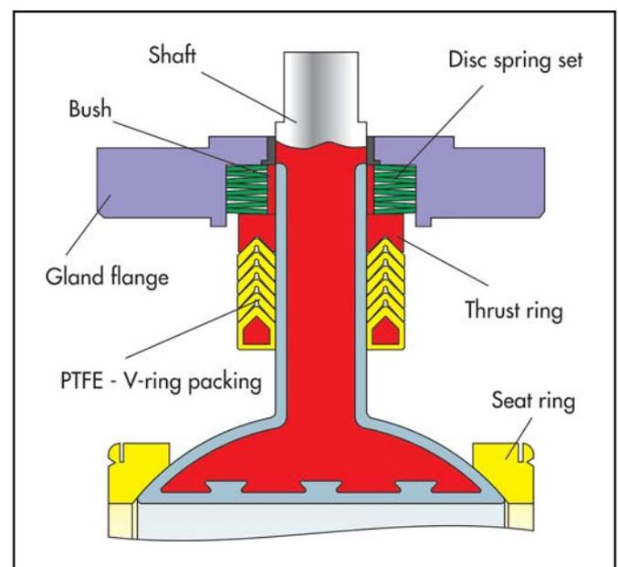
Fig. 5: Live-loaded sealing system (DIN version)
