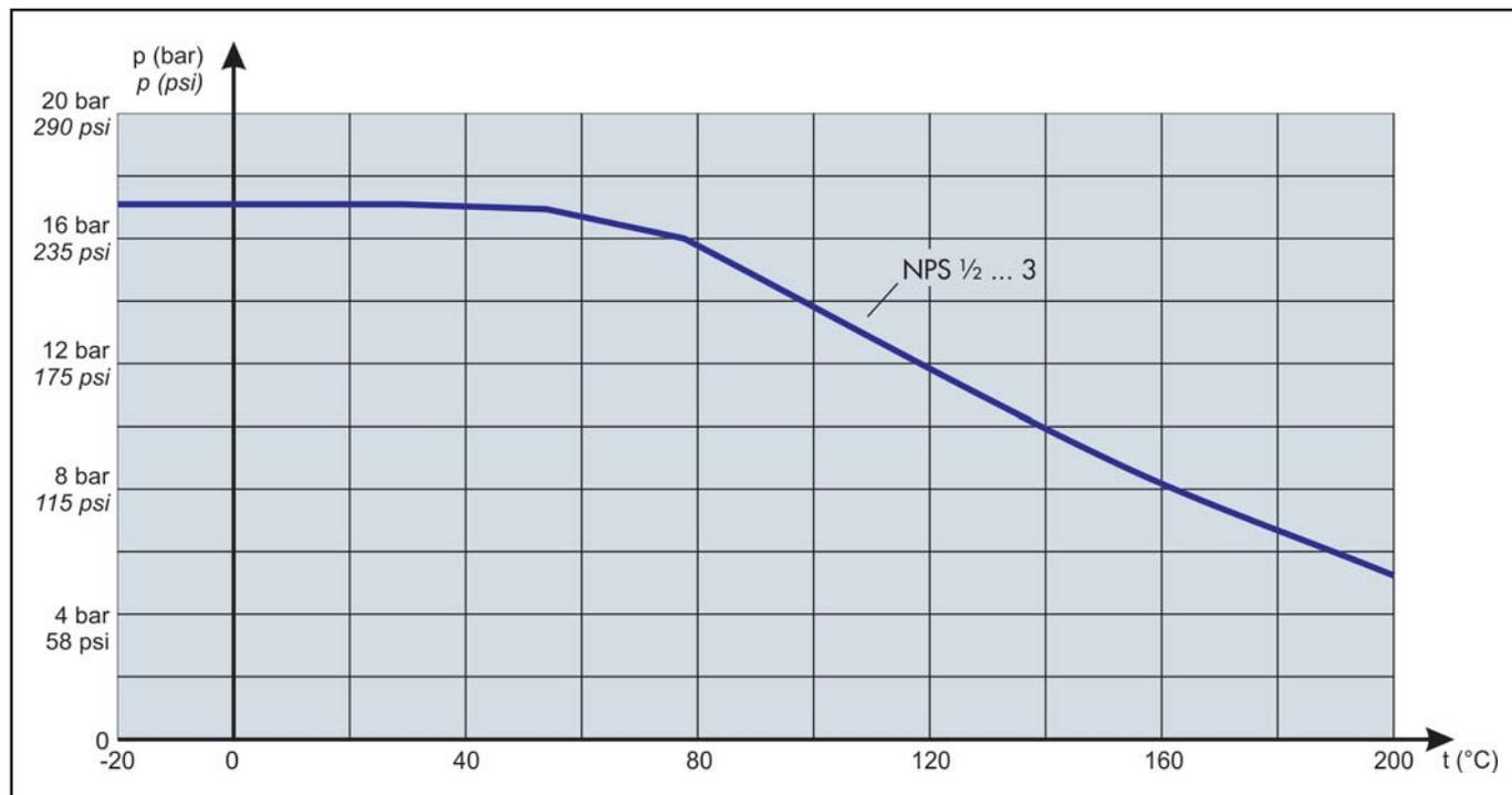
Fig. 7: Pressure-temperature diagram, c1150
