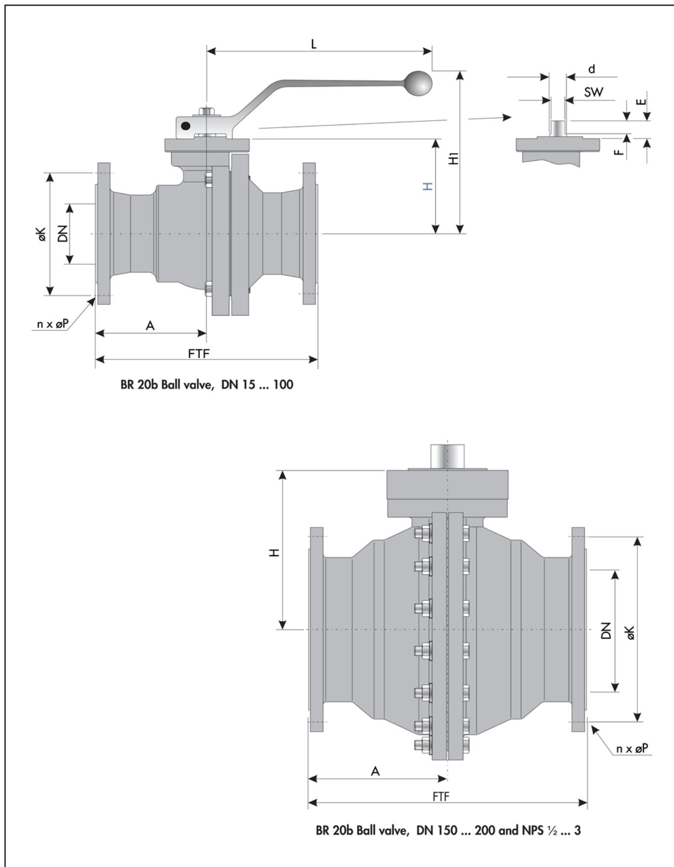
Fig. 8: Dimensional drawing of ball valve
