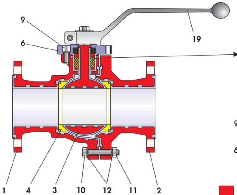
Fig 3: BR 20b Ball valve, DN 15 ... 100
