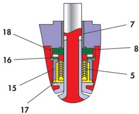
Fig 4: BR 20b Ball valve, NPS 1/2 ... 3
