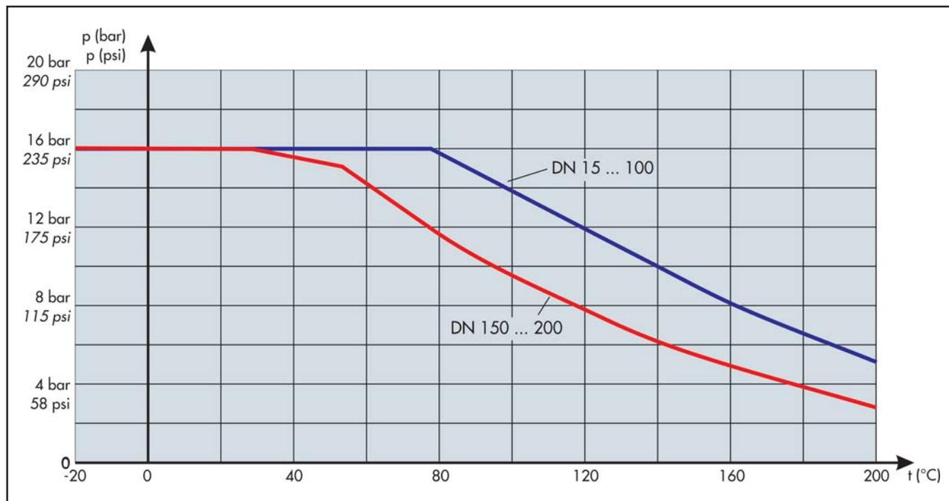
Fig. 6: Pressure-temperature diagram, PN 16
