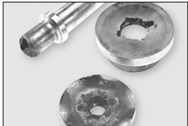
**Figure 4: Damage to Trim Parts Caused by Cavitation**
