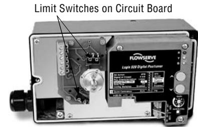
Figure 13: Position Transmitter Connection
