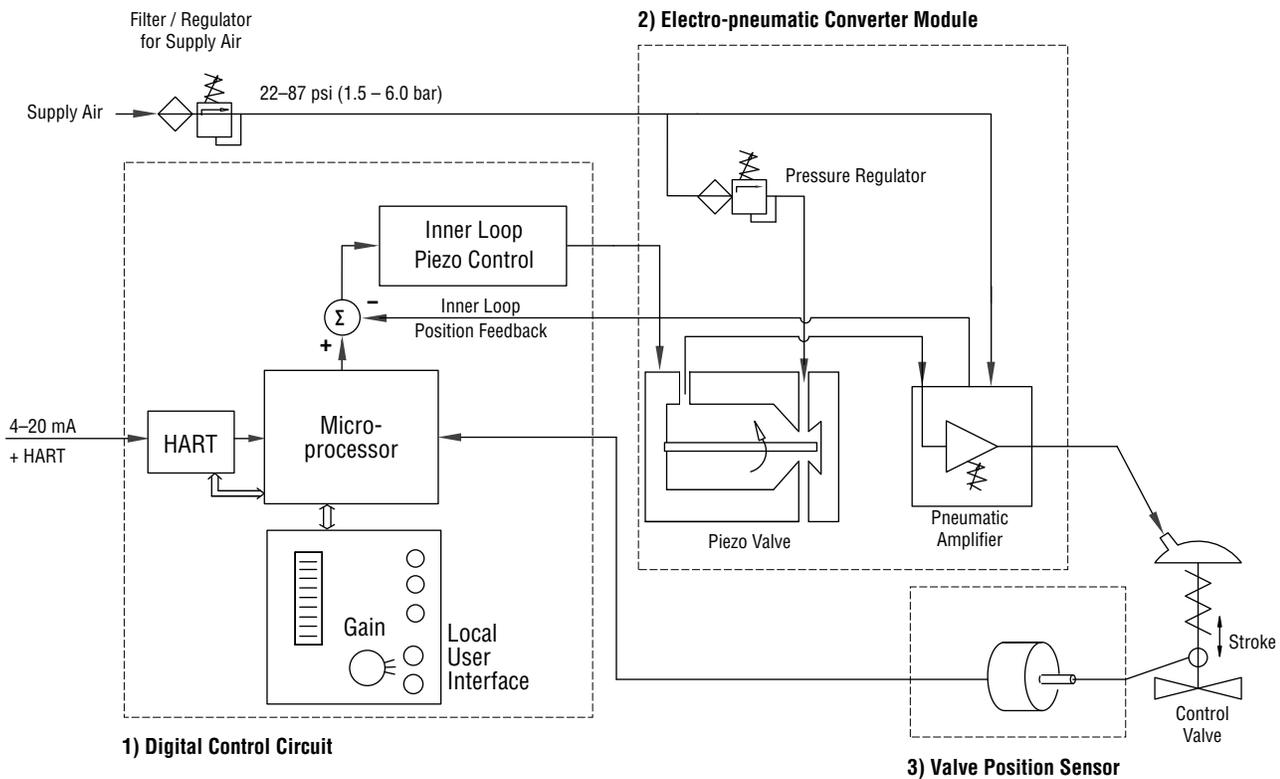
The Flowserve Logix 520si positioner is a digital positioner that incorporates the HART protocol for communication. The positioner consists of three main modules: 1) the microprocessor-based electronic control module includes HART communications and direct local user interface switches; 2) the piezo-valve-based electro-pneumatic converter module; and 3) the infinite resolution valve position sensor.
