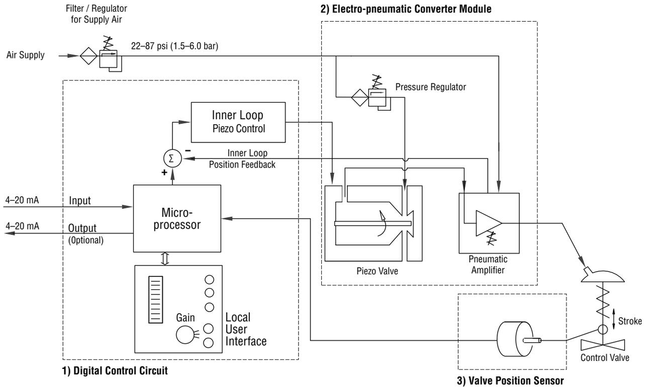
The Flowserve Logix 510si positioner is a digital positioner operated with an analog 4–20 mA input signal. The positioner consists of three main modules: 1) the microprocessor-based electronic control module with optional analog feedback and direct local user interface switches; 2) the piezo-valve-based electro-pneumatic converter module; and 3) the infinite resolution valve position sensor.
