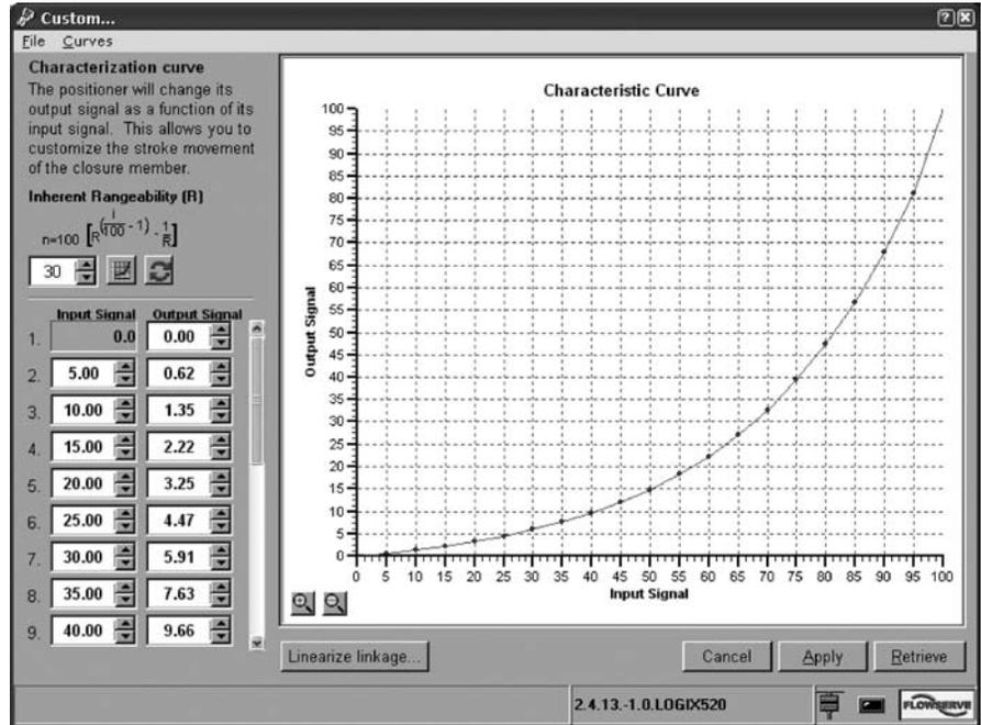
Figure 8: Manual Tuning with User Interface
