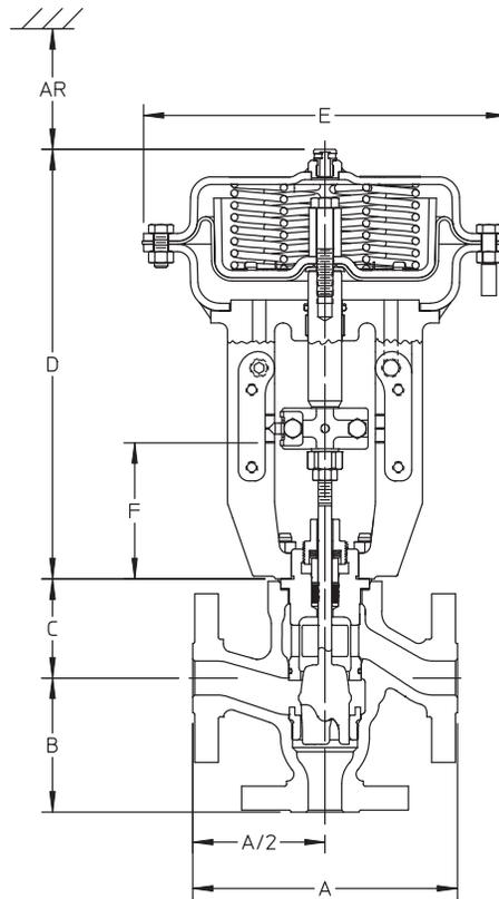
Figure 16. Fisher® GX 3-Way Dimensions (also see table 13)
