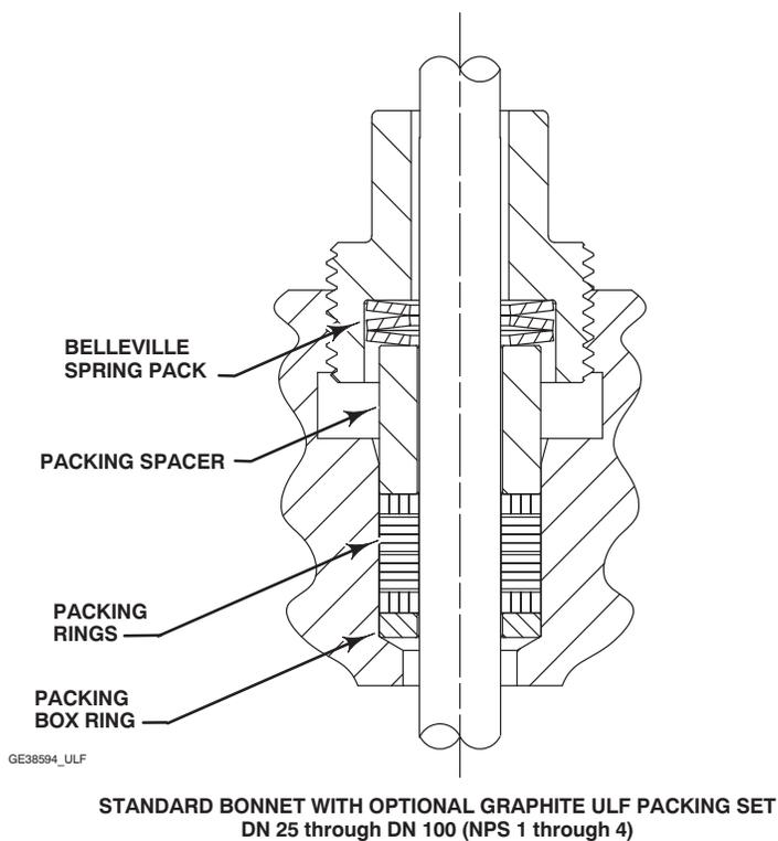
Figure 14. Fisher® GX 3-Way Packing
