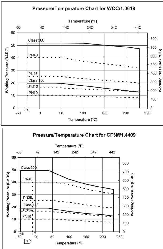
Figure 13. Material Pressure/Temperature Curves
