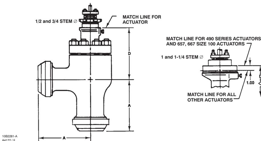
Figure 30. NPS 3 through 8 Angle Valve CL1500 Dimensions with Standard Bonnet and Style 1 Extension Bonnet (also see table 28)
