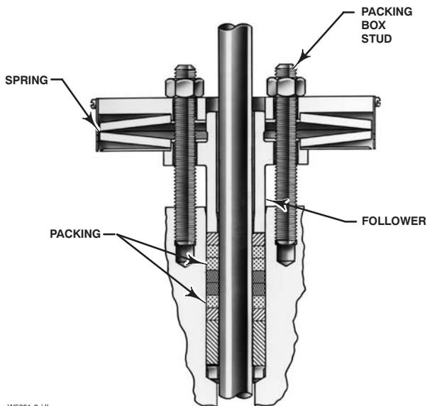
Figure 2. Typical HIGH-SEAL Packing System
