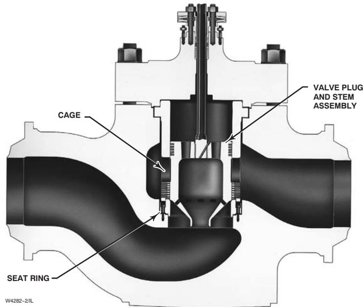
Figure 18. Sectional of NPS 20 Fisher® EHD Control Valve Assembly
