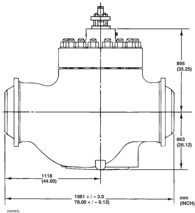
Figure 32. Dimensions (NPS 20 Fisher® EHD Valve)
