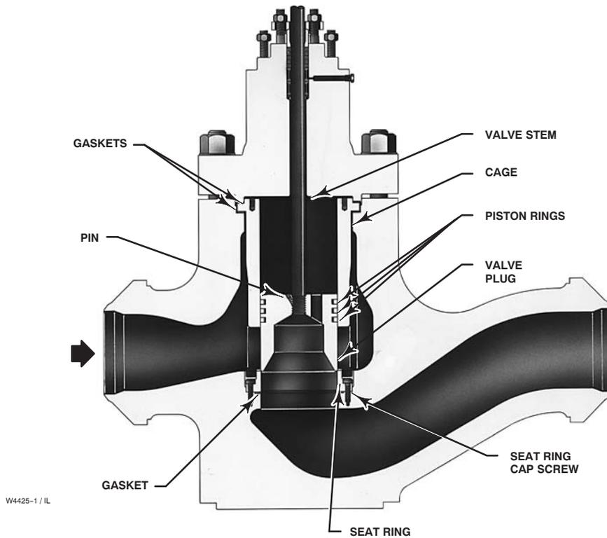
Figure 12. Fisher® EHD Valve Assembly (NPS 8 through 14 Globe Valves)
