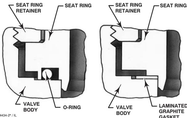
O-RING GASKET CONSTRUCTION, STANDARD CONSTRUCTION FOR EHT, CAVITROL TRIMS, AND SOUR SERVICE 1
