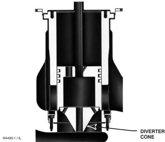
**DIVERTER CONE VALVE PLUG USED IN BOILER FEEDWATER SERVICE FOR  $\Delta P > 1000$  PSI (69 BAR) AND IN OTHER APPLICATIONS FOR  $\Delta P > 2000$  PSI (138 BAR) OR FOR WHISPER TRIM III LEVEL A, B, OR C CAGES**
