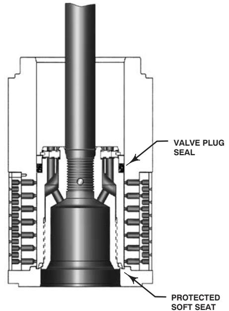
Figure 23. Typical Balanced TSO (Tight Shutoff) Trim
