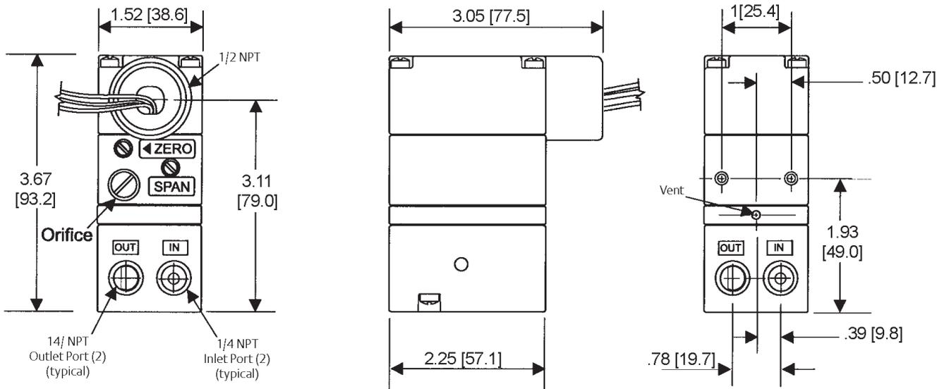
Figure 11. TA6000 Electropneumatic Transducer Dimensions, inches [millimeters]
