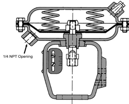
**Figure 8.** Type 16 Actuator Sectional
