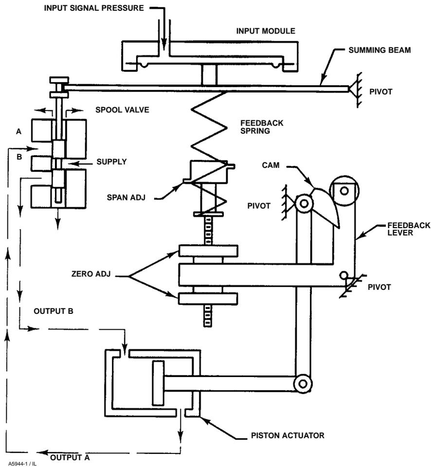
Figure 6. Fisher® 3710 Positioner Schematic
