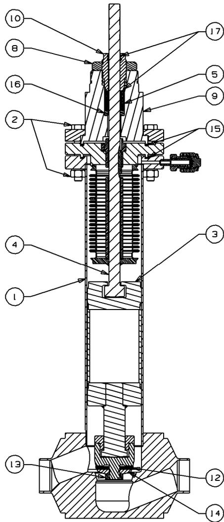
Figure 6 - Bellows Seal Automatic Valve
