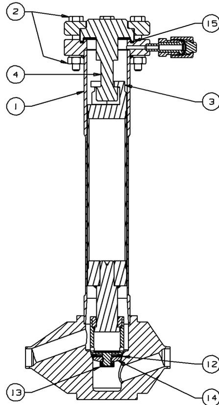
Figure 7 - Lift Check Valve
