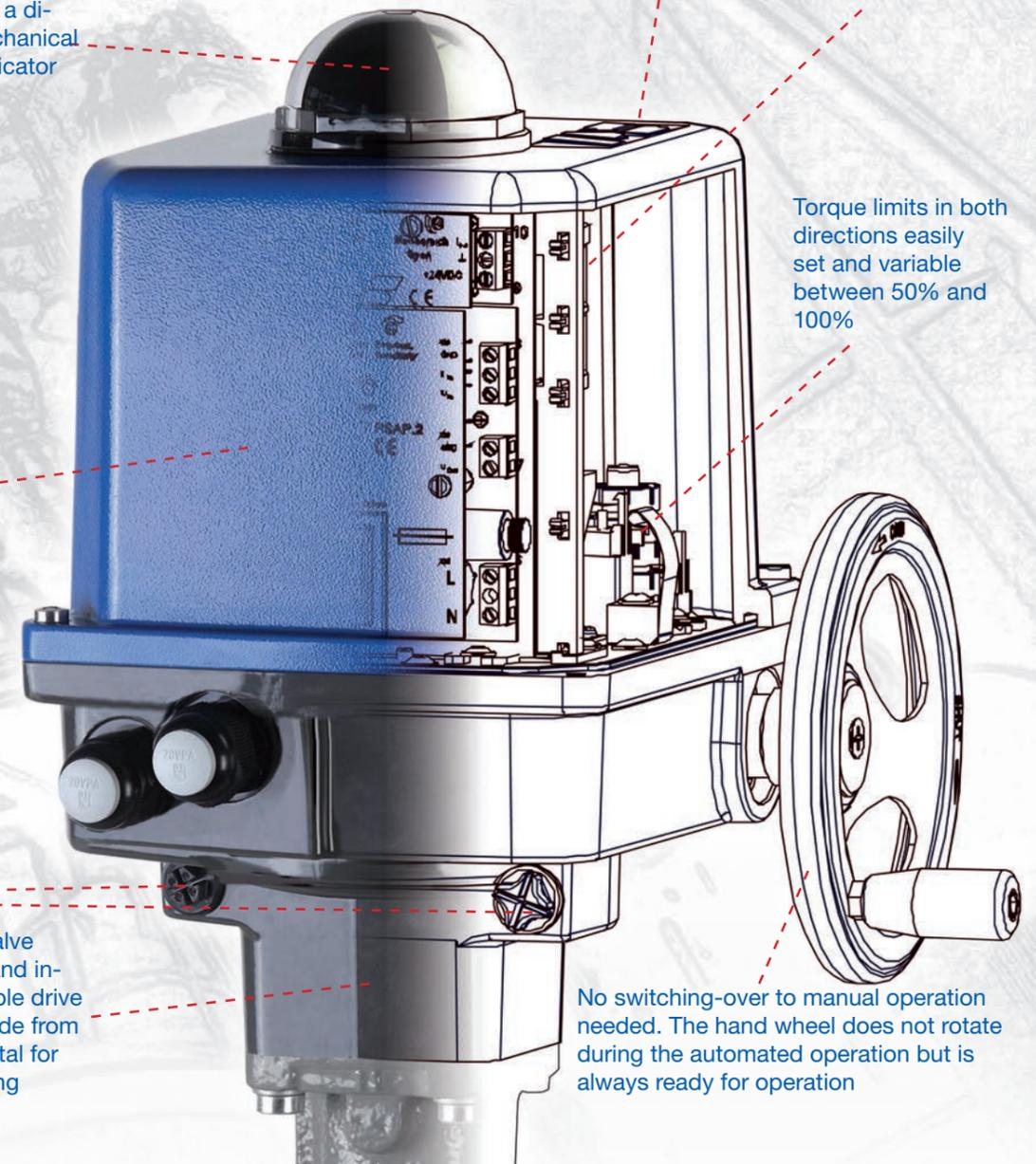
ISO 5211 valve connector and interchangeable drive bushing made from sintered metal for fast mounting
